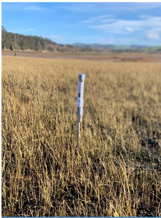
SED-sensor installed in a Spartina maritima meadow in Santander Bay.
